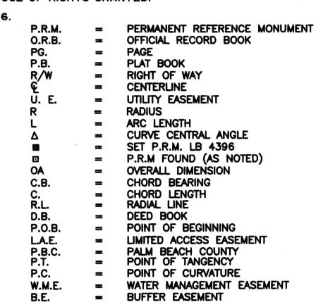
ALL BEARINGS SHOWN HEREON ARE ASSUMED TO BE NON-RADIAL UNLESS OTHERWISE NOTED AS RADIAL (R.L.).
